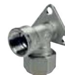
90° elbow fitting with wall bracket, female thread and plastic or multilayer pipes connections.
