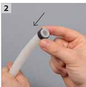
**Ring insertion.** Insert the special copper crimp ring onto the pipe.
