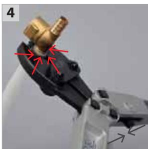
**Crimp.** Position the crimping tool so that the ring will be completely covered from its jaws. Be sure to keep the tool perpendicular to the pipe axis and close it completely.
