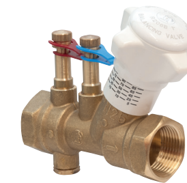
R206B | STATIC BALANCING VALVE BALANCING IS ESSENTIAL TO SAVING THE ENERGY USED IN HYDRONIC SYSTEMS. THE R206B ARE STATIC BALANCING VALVES, THAT ALLOW A GRADUAL AND PRECISE REGULATION OF THE FLOW RATE. THE R206B VALVES HAVE A FLOWMETER WITH CALIBRATED ORIFICE (VENTURI PRINCIPLE), THAT IS WITH FIXED KV. THROUGH THE PRESSURE OUTLETS (DEPENDING ON THE VERSIONS THEY ARE PROVIDED WITH OR THEY ARE OPTIONAL ACCESSORY) AND A DIFFERENTIAL MANOMETER, IT ALLOWS TO CAREFULLY MEASURE THE FLOW RATE ACTUALLY CIRCULATING.
