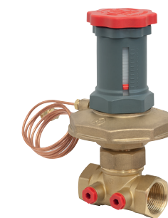
R206C | DIFFERENTIAL PRESSURE CONTROLLER R206C BALANCING VALVES CONTROL THE DIFFERENTIAL PRESSURE MAINTAINING IT CONSTANT WITH ANY FLOW. THE NOMINAL DIFFERENTIAL PRESSURE CAN BE CONTROLLED ON A CONSTANT BASIS FROM 5 TO 30 KPa IN "L" MODE (LOW) OR FROM 25 TO 60 KPa IN "H" MODE (HIGH). THE ADJUSTMENT VALUE IS SPECIFIED IN THE DIAGRAM. THE ORIGINAL FACTORY NOMINAL SET POINT IS SET TO THE MINIMUM. THE INCLUDED 1 M CAPILLARY PIPE SHOULD BE CONNECTED TO THE CIRCUIT CONTROL VALVE WITHIN THE FLOW.
